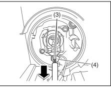
5) Pull on the cable (4) toward the rear of the vehicle to remove the bulb socket (5) from the parking light body.
